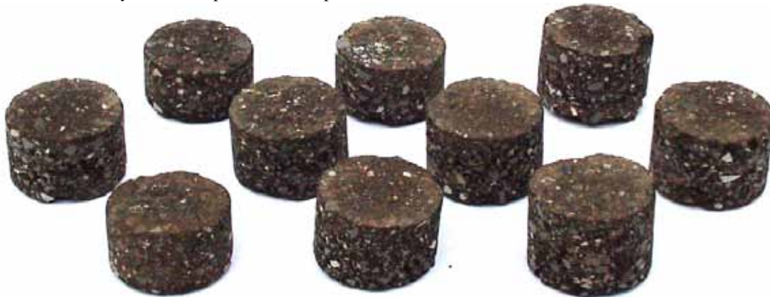
Cores Extracted from EMC SQUARED Stabilized Asphalt Millings Pavement in Gallup, New Mexico
