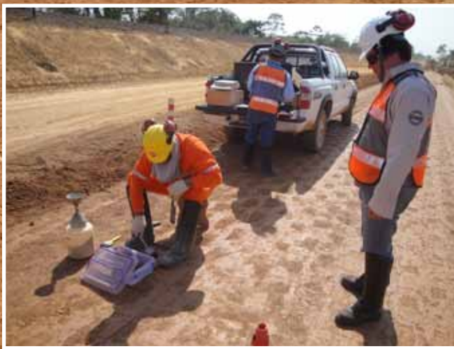
Compaction Testing of EMC SQUARED System Stabilized Subballast Layer
