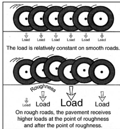
**Pavement roughness leads to higher dynamic loads on localized pavement sections that increases pavement deterioration at those locations. This lowers ride quality and leads to a cycle of increasing deterioration rates and roughness severity.**
