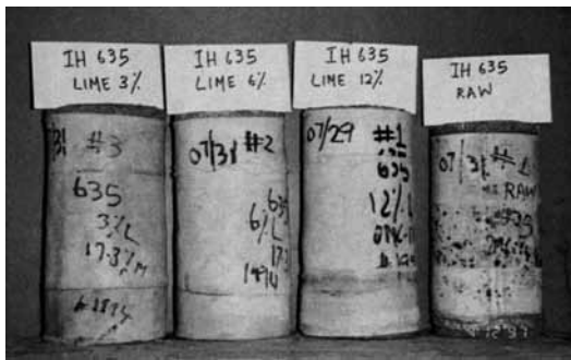
Figure 3 - Photograph Showing Comparisons of Swell (Lime vs Raw) - IH 635
