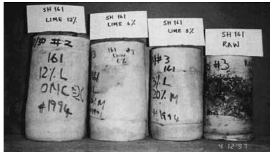
Figure 2 - Photograph Showing Comparisons of Swell (Lime vs Raw) - SH 161
